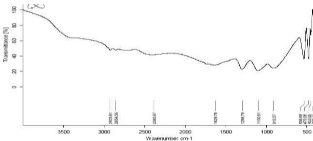
Figure.2:-Pure KDP Crystal FTIR Spectrum
