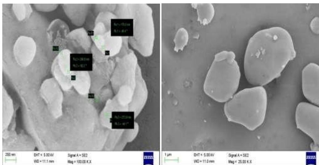
Fig.10:-SEM pattern of pure and clove doped KDP crystals
