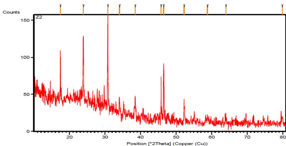
Fig.5:-Powder X-rd design of clove KDP Crystal
