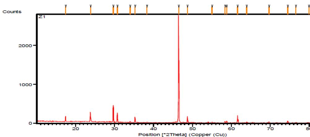
Figure. 4:-Pure KDP Crystal Powder XRD pattern
