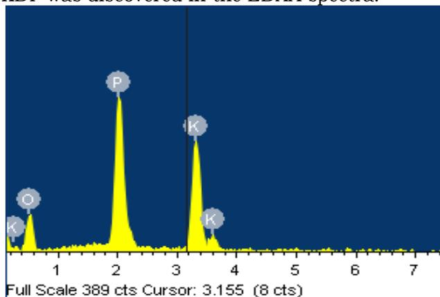
**Figure 11:- (a) Pure KDP crystal EDAX Spectrum**
