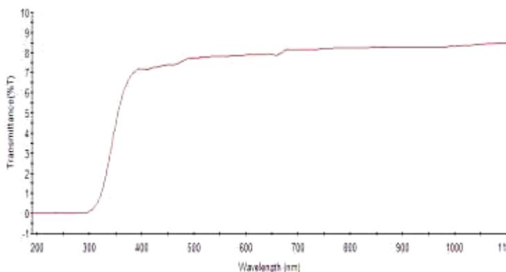
Figure.6:-Reflectance spectra of a KDP crystal doped with ginger extract
