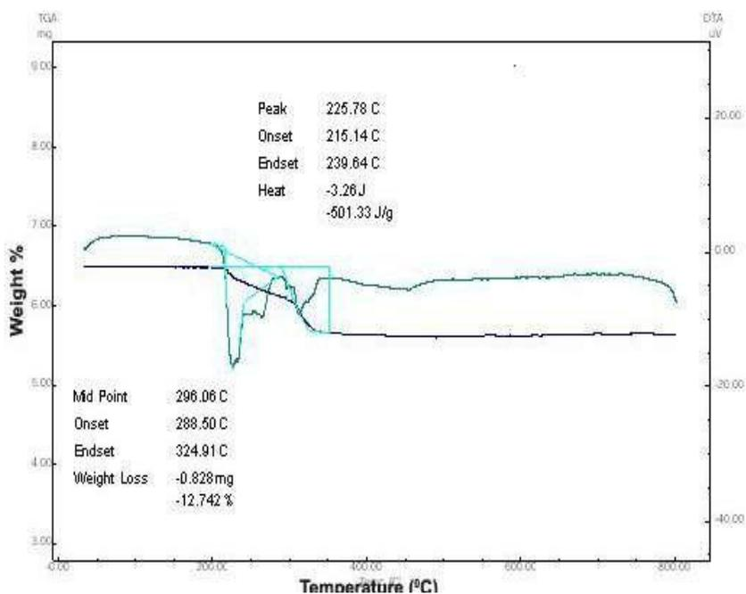
Fig.9 :-Clove doped KDP Crystal graph between TG and DTA
