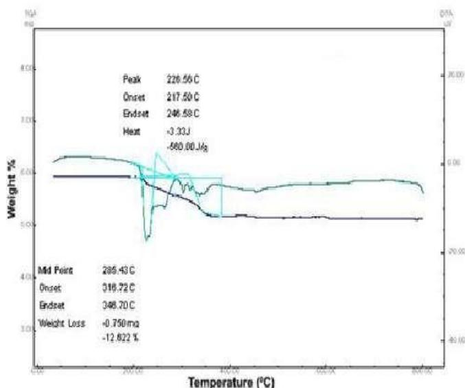
Figure 8 :-Pure KDP Crystal graph between TG and DTA
