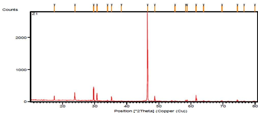
Figure. 4:-Pure KDP Crystal Powder XRD pattern
