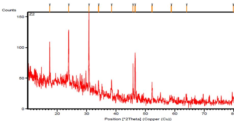
Fig.5:-Powder X-rd design of clove KDP Crystal
