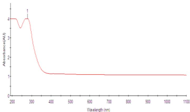
Figure.7:-Ginger extract doped KDP crystal absorbance spectra.
