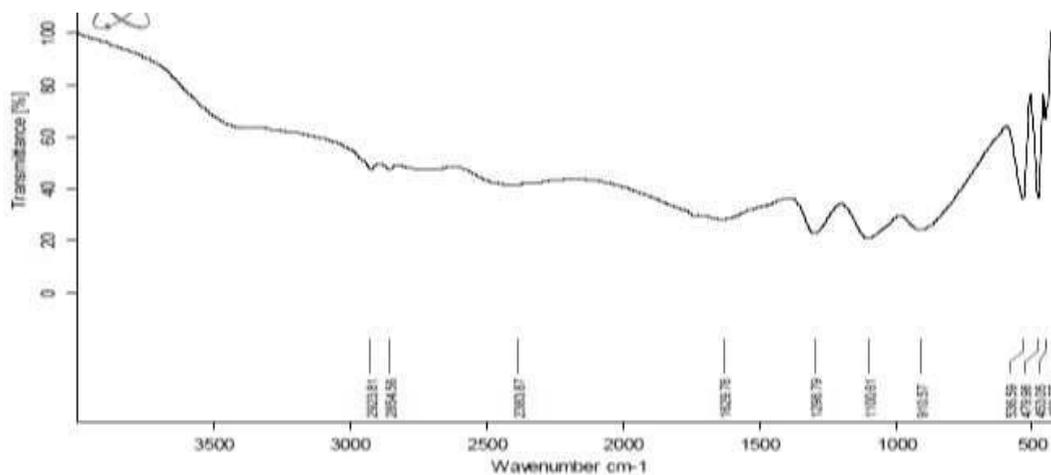
Figure.2:-Pure KDP Crystal FTIR Spectrum
