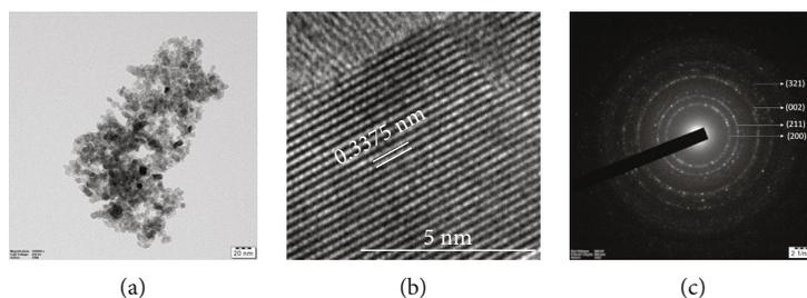
FIGURE 5: (a) HRTEM image, (b) HRTEM lattice image, and (c) SAED pattern obtained from the 0.05 M Fe-SnO<sub>2</sub> NPs.
