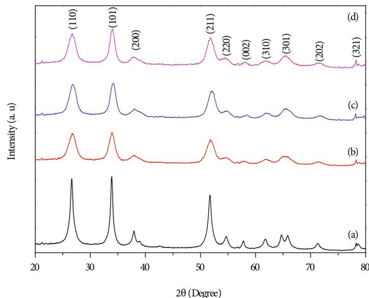
FIGURE 1: XRD patterns of (a) pure, (b) 0.01 M, (c) 0.03 M, and (d) 0.05 M Fe-SnO<sub>2</sub> NPs.
