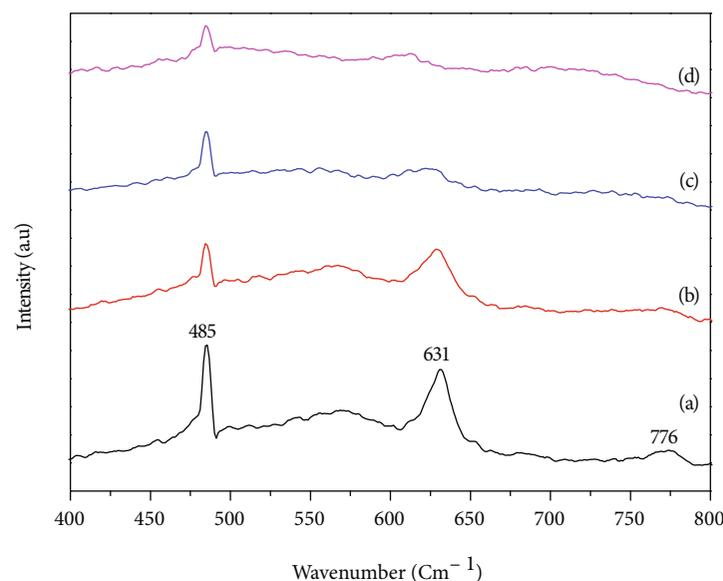
FIGURE 2: Raman spectra of (a) pure, (b) 0.01 M, (c) 0.03 M, and (d) 0.05 M Fe-SnO<sub>2</sub> NPs.
