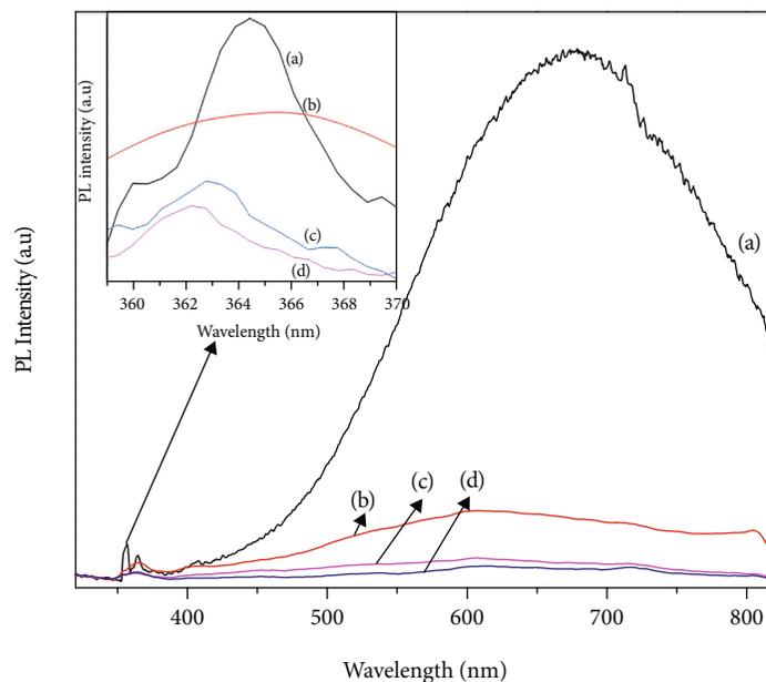
FIGURE 7: PL spectra of (a) pure, (b) 0.01 M, (c) 0.03 M, and (d) 0.05 M Fe-SnO<sub>2</sub> NPs.
