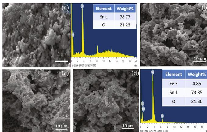
FIGURE 4: SEM micrographs of (a) pure, (b) 0.01 M, (c) 0.03 M, and (d) 0.05 M Fe-SnO<sub>2</sub> NPs and EDS spectra of pure and 0.05 M Fe-SnO<sub>2</sub> NPs.
