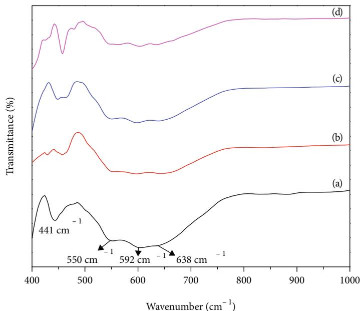
FIGURE 3: FTIR spectra of (a) pure, (b) 0.01 M, (c) 0.03 M, and (d) 0.05 M Fe-SnO<sub>2</sub> NPs.
