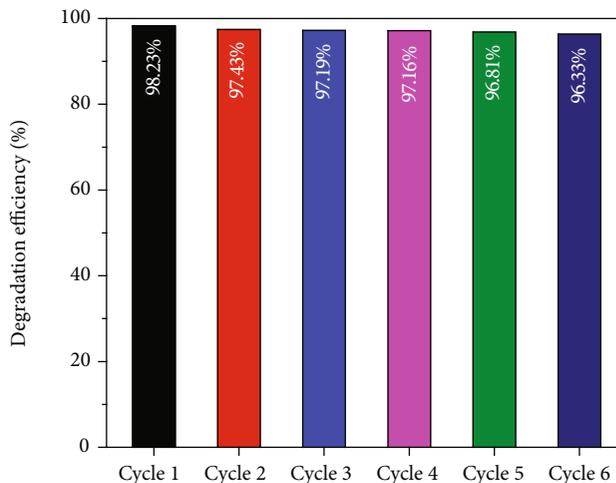
FIGURE 11: Recycling ability and stability of 0.05 M Fe-SnO<sub>2</sub> nanoparticles.
