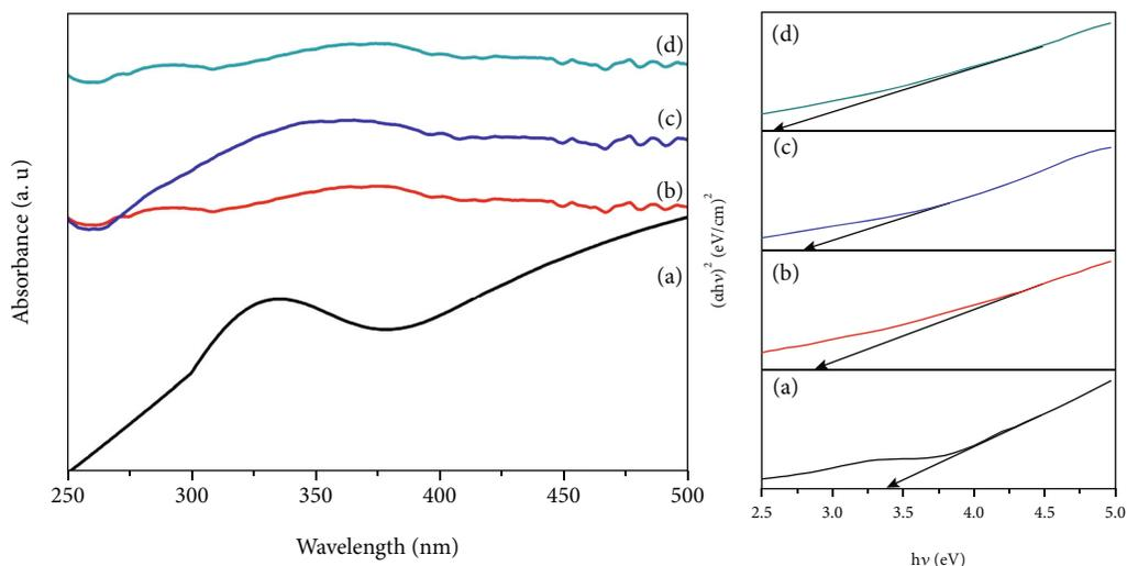
FIGURE 6: Optical absorption spectra and Tauc's plot of (a) pure, (b) 0.01 M, (c) 0.03 M, and (d) 0.05 M Fe-SnO<sub>2</sub> NPs.
