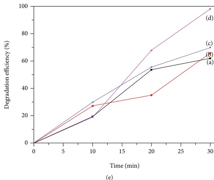
FIGURE 8: Optical absorption spectra depicting the degradation of crystal violet dye using (a) pure, (b) 0.01 M, (c) 0.03 M, (d) 0.05 M Fe-SnO<sub>2</sub> NPs, and (e) efficiency vs. time graph.
