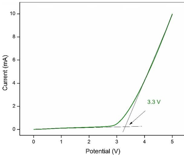
**Fig. 10** Linear sweep voltammetry of highest conducting polymer electrolyte
