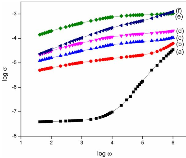
**Fig. 6** Conductance spectra of (a) pure P(VdCl...), (b) 70 wt% P(VdCl...):30 wt% MgCl<sub>2</sub>, (c) 70 wt% P(VdCl...): 30 wt% MgCl<sub>2</sub>: 0.1 wt% SN, (d) 70 wt% P(VdCl...): 30 wt% MgCl<sub>2</sub>: 0.2 wt% SN, (e) 70 wt% P(VdCl...): 30 wt% MgCl<sub>2</sub>: 0.3 wt% SN, (f) 70 wt% P(VdCl...): 30 wt% MgCl<sub>2</sub>: 0.4 wt% SN
