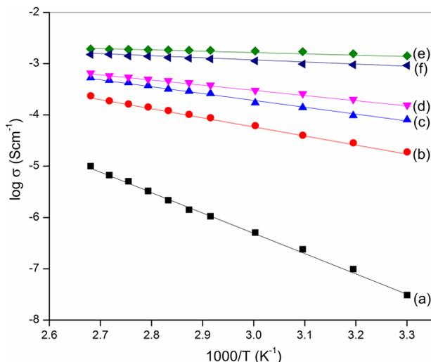
**Fig. 7** Arrhenius plot of (a) pure P(VdCl...), (b) 70 wt% P(VdCl...):30 wt% MgCl<sub>2</sub>, (c) 70 wt% P(VdCl...): 30 wt% MgCl<sub>2</sub>: 0.1 wt% SN, (d) 70 wt% P(VdCl...): 30 wt% MgCl<sub>2</sub>: 0.2 wt% SN, (e) 70 wt% P(VdCl...): 30 wt% MgCl<sub>2</sub>: 0.3 wt% SN, (f) 70 wt% P(VdCl...): 30 wt% MgCl<sub>2</sub>: 0.4 wt% SN
