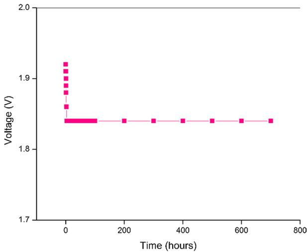
**Fig. 12** Discharge characteristics of primary battery through 100 KΩ (Mg | SPE | MnO<sub>2</sub> cathode)
