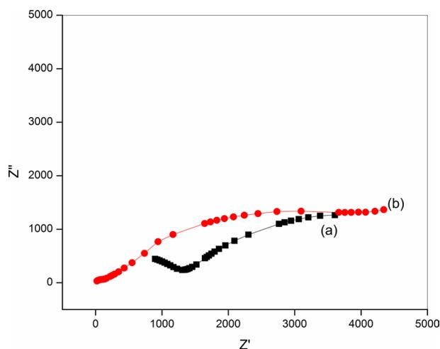
**Fig. 9** Impedance plot of Mg | SPE | Mg cell (a) before polarization and (b) after polarization
