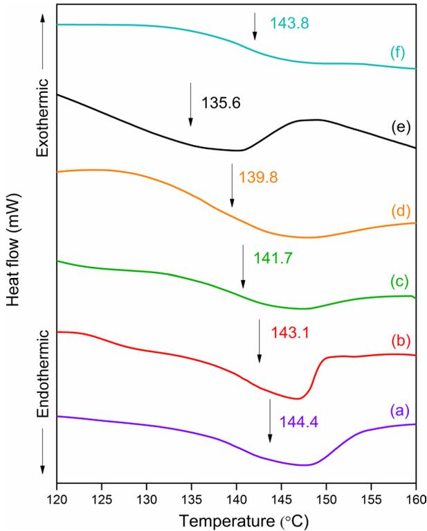
**Fig. 3** DSC curves of (a) pure P(VdCl...), (b) 70 wt% P(VdCl...):30 wt% MgCl<sub>2</sub>, (c) 70 wt% P(VdCl...): 30 wt% MgCl<sub>2</sub>; 0.1 wt% SN, (d) 70 wt% P(VdCl...): 30 wt% MgCl<sub>2</sub>; 0.2 wt% SN, (e) 70 wt% P(VdCl...): 30 wt% MgCl<sub>2</sub>; 0.3 wt% SN, (f) 70 wt% P(VdCl...): 30 wt% MgCl<sub>2</sub>; 0.4 wt% SN
