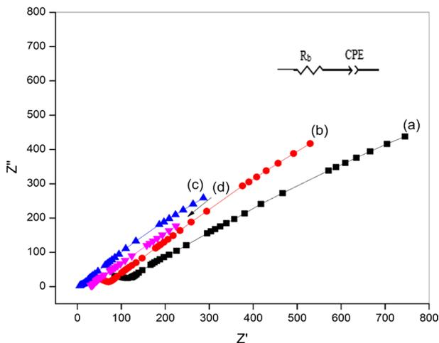
**Fig. 5** Nyquist plot of (a) 70 wt% P(VdCl...): 30 wt%  $MgCl_2$ : 0.1 wt% SN, (b) 70 wt% P(VdCl...): 30 wt%  $MgCl_2$ : 0.2 wt% SN, (c) 70 wt% P(VdCl...): 30 wt%  $MgCl_2$ : 0.3 wt% SN and (d) 70 wt% P(VdCl...): 30 wt%  $MgCl_2$ : 0.4 wt% SN**Table 3** Conductivity values of plasticized polymer electrolytes calculated from Nyquist plot
