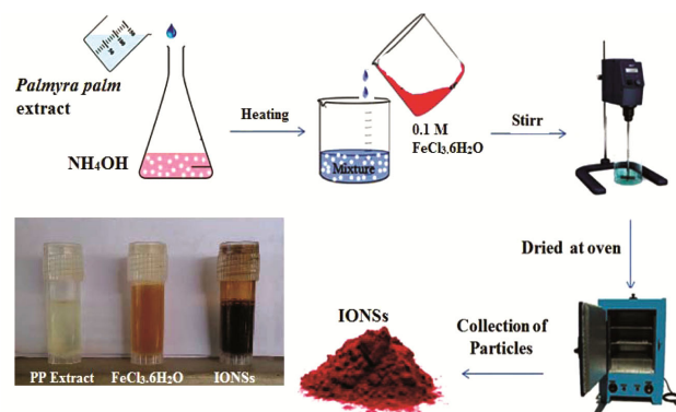
Fig. 1 — Scheme of preparation of Iron oxide nanopindles (IONSs)
