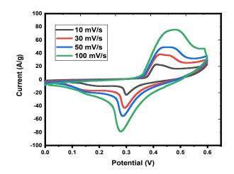
Fig. 6. CV studies of Cu-ZnO prepared by the green synthesis using maize
