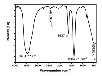
Fig. 1. FTIR spectra of Cu-ZnO prepared by the green synthesis using maize
