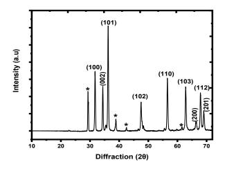
Fig. 2. Diffraction pattern of Cu-ZnO prepared by the green synthesis using maize
