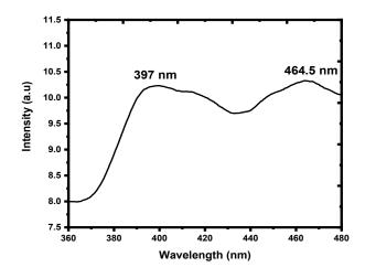
Fig. 5. PL spectra of Cu-ZnO prepared by the green synthesis using maize
