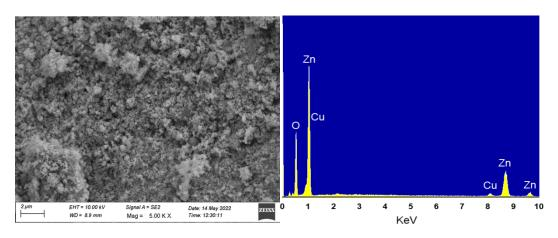
Fig. 3. SEM and EDS spectra of Cu-ZnO prepared by the green synthesis using maize
