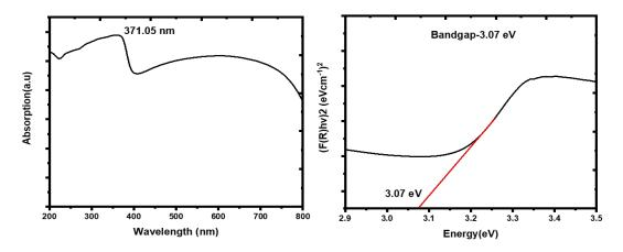
Fig. 4. Absorption and bandgap spectra of Cu-ZnO prepared by the green synthesis using maize
