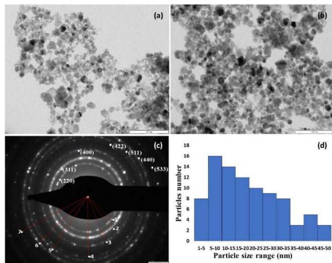
**Fig. 2** TEM analysis of Chi-Fe<sub>3</sub>O<sub>4</sub> nanocomposites
