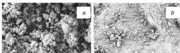
**Fig. 3** FESEM analysis of Chi-Fe<sub>3</sub>O<sub>4</sub> nanocomposites
