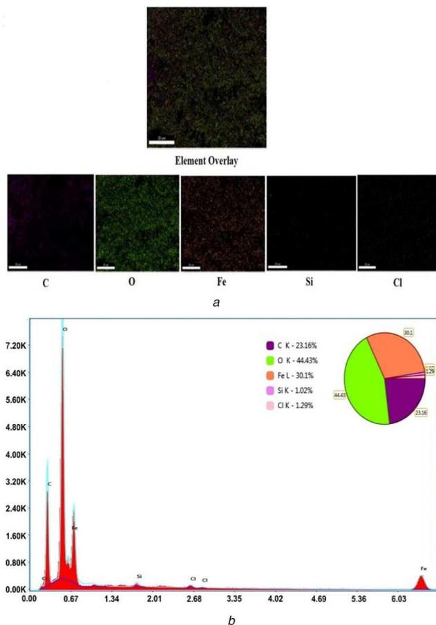
**Fig. 4** EDS analysis and elemental mapping (a) Elemental mapping, (b) EDS analysis of Chi-Fe<sub>3</sub>O<sub>4</sub> nanocomposites
