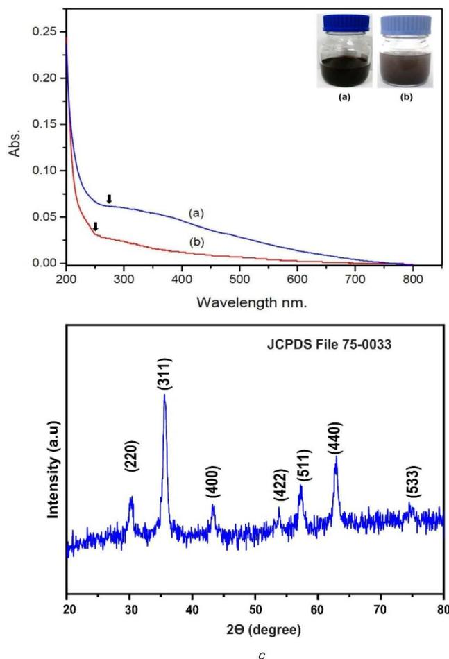
**Fig. 1** UV-Vis spectrum of Chi-Fe<sub>3</sub>O<sub>4</sub> nanocomposites
