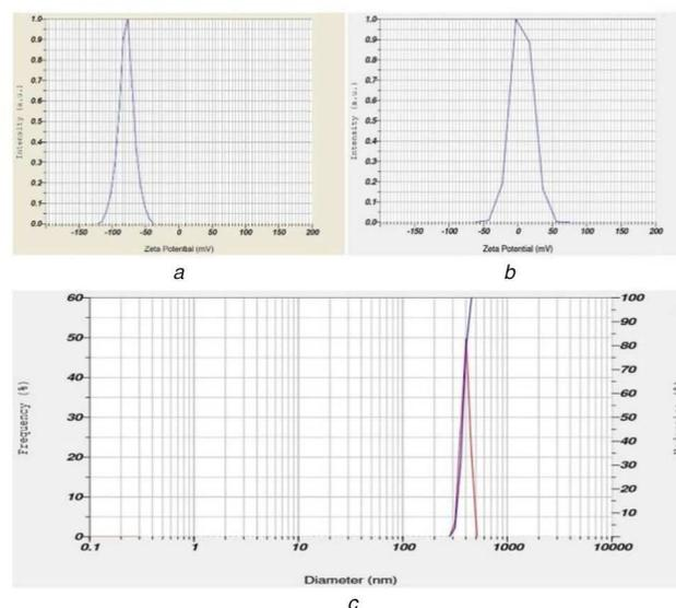
**Fig. 6** Zeta potential and DLS analysis (a) Zeta potential analysis of Fe<sub>3</sub>O<sub>4</sub>, (b) Zeta potential analysis of Chi-Fe<sub>3</sub>O<sub>4</sub> nanocomposites, (c) DLS studies of Chi-Fe<sub>3</sub>O<sub>4</sub> nanocomposites
