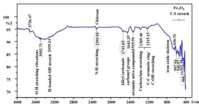
**Fig. 5** FTIR analysis of Chi-Fe<sub>3</sub>O<sub>4</sub> nanocomposites
