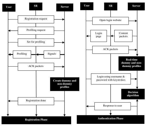
Fig.1: Extended CLAS Authentication Flowchart
