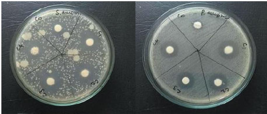
**Figure 8.** Bactericidal study of Mn doped ZnO nanoparticles against *S. aureus* and *B. subtilis*.
