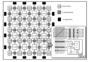
Figure 2. FPGA Architecture.
