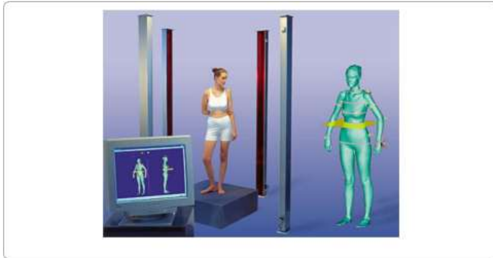
Fig. 1 3D body scanning by Laser scanner
