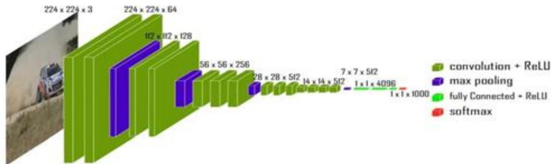
Figure 4: VGG16 Architecture (Image source: [35])
