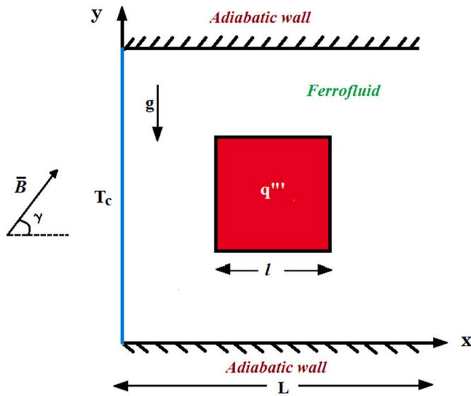
Fig. 1. Physical geometry.
