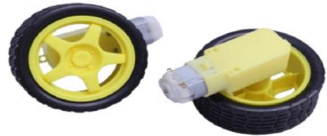
Figure : 2 DC Motors used in this System
