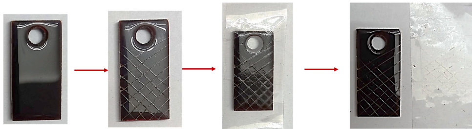
Fig. 7. Crosscut test of THQ-PBZ coated MS plate.
