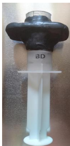
Figure 4. The overall completed apparatus setup with tissue loaded barrel with plunger. Freshly excised chicken heart inserted into the barrel from the rear end.
