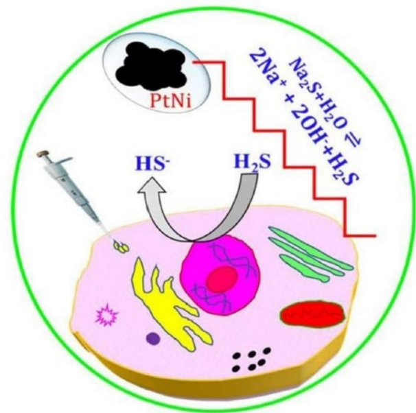
Fig. 9 Schematic representation of an electrochemical sensing platform using PtNi nanoparticles for the detection of hydrogen sulfide emissions in breast cancer cells (reproduced from [100] with permission from MDPI under CC by 4.0 license)
